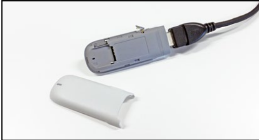
Insert sim-card into USB modem
